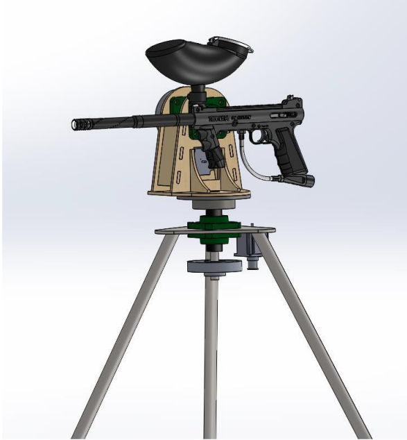
Fig. 1. An overview of the structure of the Motion-Detecting Sentry Turret. The chassis will house most of the hardware components.
